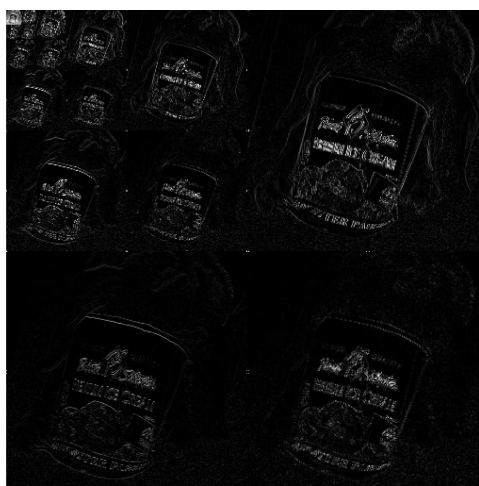
Figure 2: The result of applying the Haar wavelet transform recursively to the upper left bin.
