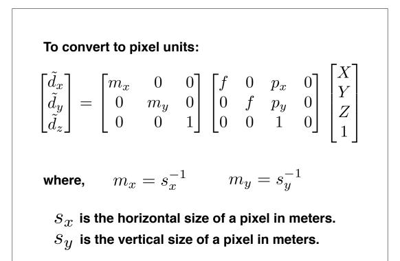
$$\begin{bmatrix} \tilde{d}_x \\ \tilde{d}_y \\ \tilde{d}_z \end{bmatrix} = \begin{bmatrix} m_x & 0 & 0 \\ 0 & m_y & 0 \\ 0 & 0 & 1 \end{bmatrix} \begin{bmatrix} f & 0 & p_x & 0 \\ 0 & f & p_y & 0 \\ 0 & 0 & 1 & 0 \end{bmatrix} \begin{bmatrix} X \\ Y \\ Z \\ 1 \end{bmatrix}$$
