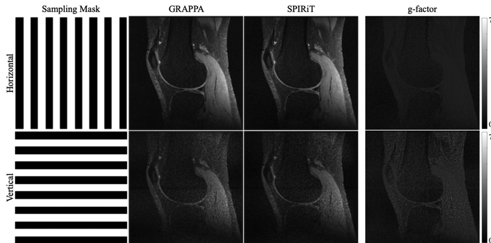
Fig. 4 Reconstructions of sagittal slices of a knee with different sampling patterns. The columns from left to right are a representation of the sampling indicating the undersampling direction, the GRAPPA reconstruction, the SPIRiT reconstruction, and the g-factor of the SPIRiT reconstructions. The top and bottom rows show undersampling in the horizontal (anterior-posterior) and vertical (superior-inferior) directions, respectively. Both sampling masks used a reduction factor of 2. All reconstructions used a 31 \times 31 FSR and a 3 \times 3 kernel.
